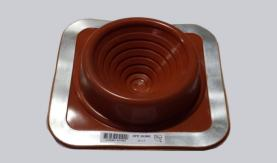
Used to seal Flue Pipe and available in 2 sizes from 75mm to 175mm and 150mm to 350mm diameters. Black dektites can be painted with acrylic paint & withstand temperature up to 115°C or 150°C intermittently. Red silicone dektites will withstand temps up to 200°C or 250°C intermittently with a BAL rating of 29. Low profile base with watershed sleeve Large square base will cover a larger opening. Twenty Year warranty – just fit it and forget it! CSA Approval number 70029509
