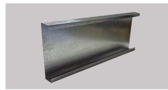
A cover made to conceal flue pipe that exits the back of a heater and up a wall. Standard sizes 350 x 70 x 900 Long and 350 x 70 x 2400 Long. Manufactured using AS/NZ Standard Grade Z275 0.6mm Galvanized Steel. Special sizes made to order.
