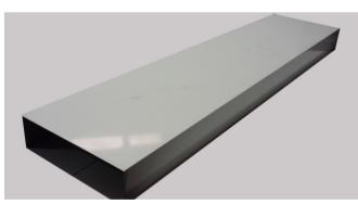
Single Skin Rectangular Flue Pipe, 285x85 available in 1200 or 2400 lengths. Manufactured using AS/NZ Standard Grade Z275 0.6mm Galvanized Steel, AS/NZ Standard 304 2b Brushed Stainless Steel or Sign White Color Bond.
