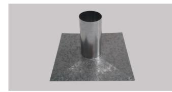
AUSTRALIA \* \* \* Various sized Chimney Plates from 100mm diameter Flue x 150H x 350 sq base up to 250mm diameter. Used to cover the outlet of a Brick or Masonry Chimney and allow the Flue Pipe to terminate using an AGA Approved Gas Cowl. Comes in 2 pieces for ease of transport. Manufactured using AS/NZ Standard Grade Z275 0.6mm Galvanized Steel.
