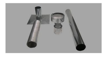
Flex Flue Kit containing 100 diameter, 125mm diameter or 150mm diameter Flexible Flue Pipe, a connector, a length of 900mm long Rigid Flue Pipe, Chimney Plate and an AGA approved Gas Cowl. Flexible Flue Pipe is Manufactured of 8006 grade Aluminium coil and the other components are manufactured using AS/NZ Standard Grade Z275 0.6mm Galvanized Steel.
