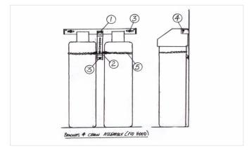
Brackets and chains to retain 2 LPG Cylinders against a wall to prevent accidentally falling over. The Hood is used to keep rain and sun off the Cylinders. Can be Powder Coated at extra cost. Manufactured using AS/NZ Standard Grade Z275 0.6mm Galvanized Steel.
