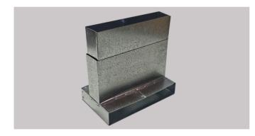
Elbow used to divert rectangle single skin flue (250mm x 40mm) through a double brick wall and up the outside of the brick wall. Manufactured using AS/NZ Standard Grade Z275 0.6mm Galvanized Steel.
