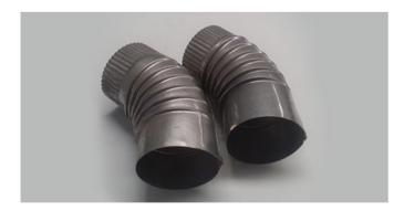
AUSTRALIA \*\*\* Used to divert round single skin flue around an obstruction. Made from 75mm diameter up to 150mm diameter x 45° and 90°, the 316 grade Stainless Steel Crimp Bends are formed to shape. Manufactured using AS/NZ Standard Grade 316 0.6mm Stainless Steel.
