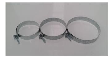
Manufactured to suit 100mm diameter up to 300mm diameter twin skin round flue pipe. Manufactured using AS/NZ Standard Grade Z275 0.6mm Galvanized Steel.
