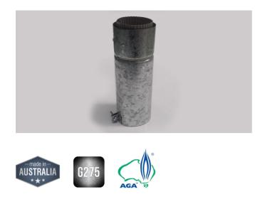
Available in 100mm diameter up to 300mm diameter x 300mm long. Manufactured using AS/NZ Standard Grade Z275 0.6mm Galvanized Steel and Aluminium inner. AGA 7715 Certification.
