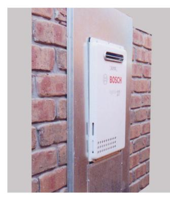
Units built into brick walls and replacing them with a standard continuous flow hot water service. Suitable for Rinnai, Rheem and Bosch systems. Come in 2 sizes, 1200 x 600 and 1800 x 600. Cover plate is supplied. Manufactured using AS/NZ Standard Grade Z275 0.6mm Galvanized Steel. Can be powder coated as needed.
