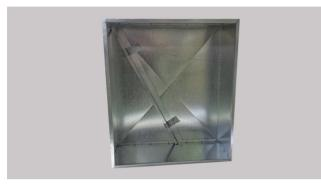
Bent up to cover up holes in the wall of removed appliances. Standard size is 900 x 900 x 80 and Manufactured using AS/NZ Standard Grade Z275 0.6mm Galvanized Steel. Special sizes made to order.
