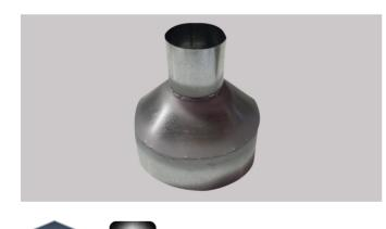
Various size Reducers to suit Single Skin Flue Pipe of the following sizes, 125mm diameter – 100mm diameter, 150mm diameter – 100mm diameter and 150mm diameter – 125mm diameter. Manufactured using AS/NZ Standard Grade Z275 0.6mm Galvanized Steel.
