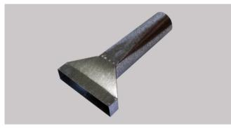
Formed metal component that adapts Twin Skin and Single Skin Rectangular flue To 100mm diameter flue pipe. Manufactured using AS/NZ Standard Grade Z275 0.6mm Galvanized Steel.
