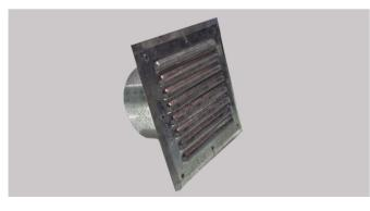
Designed to terminate round flue pipe at the wall. Comes in 100 dia. Spigot up to 200 dia. Spigot in increments of 25mm. Manufactured using AS/NZ Standard Grade Z275 0.6mm
