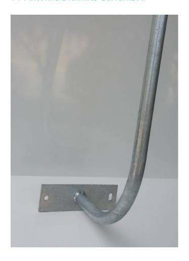
Used to extend the height of an aerial for better TV reception. Water proof with plastic cap. Fascia mounted with adjustable slot in one end and round hole in the other to level. Manufactured using AS/NZ Standard Grade Hot Dipped Galvanized Steel pipe.
