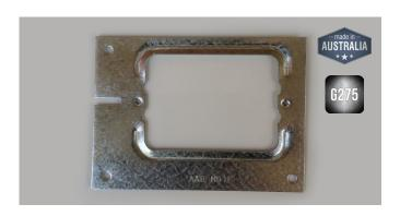
Designed simply to be nailed directly to a stud or noggin horizontally or vertically and mount a switch plate or socket. Manufactured using AS/NZ Standard Grade Z275 Galvanized Steel.
