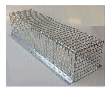
Bolted using dyna bolts or screwed and used to protect wall mounted flood lights or any light/fitting from vandalism or accidental damage. Manufactured using AS/NZ Standard Grade Mesh Steel and Hot Dipped Galvanized or Powder Coated.
