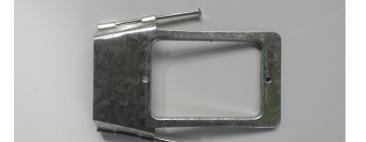
Designed to be nailed directly to a stud or noggin horizontally or vertically and mount a switch plate or socket. Manufactured using AS/NZ Standard Grade Z275 Galvanized Steel.
