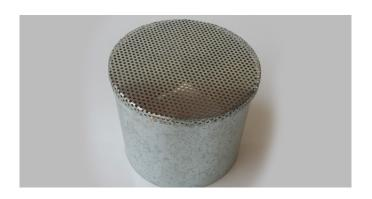
Keep fibre glass bat roof insulation from touching hot down lights. Maybe fitted to existing installation without the need to disconnect wiring. Can be retro fitted over any down light not exceeding 100dia and 100h. Manufactured using AS/NZ Standard Grade Z275 Galvanized Steel and perforated galvanized steel cover to AS/NZ 3000:2007 Wiring rules clause 4.5.2.
