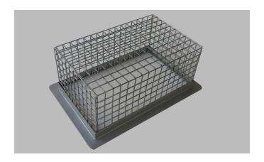
Bolted using dyna bolts or screwed and used to protect floor mounted flood lights or any light/fitting from vandalism or accidental damage. Manufactured using AS/NZ Standard Grade Mesh Steel and Hot Dipped Galvanized or Powder Coated.
