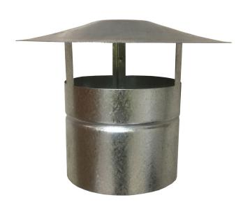
Manufactured as a non-AGA approved terminal for the ventilation of Wood Fire flue pipe. Galvanized Wood Fire Cowls without skirts are generally used for single skin wood fire situations. Come in sizes from 100mm to 250mm diameters. Can add mesh for bush fire embers protection.
