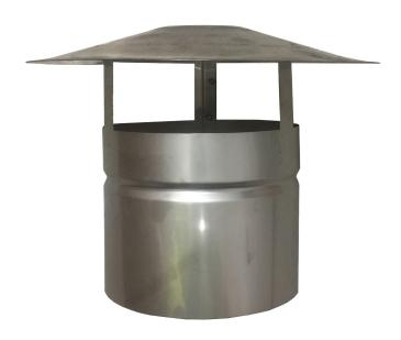
Manufactured as a non-AGA approved terminal for the ventilation of Wood Fire flue pipe. Stainless Steel Wood Fire Cowls without a skirt are generally used for single skin Wood Fire situations in a corrosive or near ocean environment. Can add mesh for bush fire embers protection. Come in sizes from 100mm to 250mm diameters.
