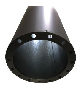
The Ceiling Box End Caps are fitted to a 900L Galvanized Outer Flue Pipe to make a Ceiling Drop Box which is then fixed to Angles that support the Ceiling Box/Flue to the roof beams. These are painted Metallic Black.
