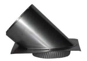
A 150mm (6") 304 2b Stainless Steel 45-degree Wood Fire direct offset is for diverting the pipe to  $45^\circ$ . It can be installed on roofs and or floors.
