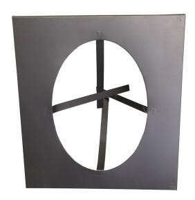
Ceiling Flange is used to neaten up the cut out and help provide clearance in the ceiling for the flue pipe or ceiling box to pass through. Designed in an elliptical shape to match the outside of a flue passing through a Raked ceiling of various angles from 10 degrees up to 30 degrees.. Can be made in various flue sizes from 75mm diameter up to 300mm.
