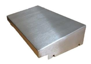
30 degree sloping roof for self-draining manufactured in 1 piece and bolts to existing Economy Enclosure using blind nut-serts to retain PI rating of IP65. Manufactured in Galvanized Z275 Steel, Powder Coated and 304 and 316 #4 Stainless Steel.
