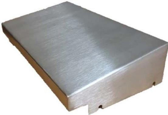
30 degree sloping roof for self-draining manufactured in 1 piece and bolts to existing Economy Enclosure using blind nut-serts to retain PI rating of IP65. Manufactured in Galvanized Z275 Steel, Powder Coated and 304 and 316 #4 Stainless Steel.
